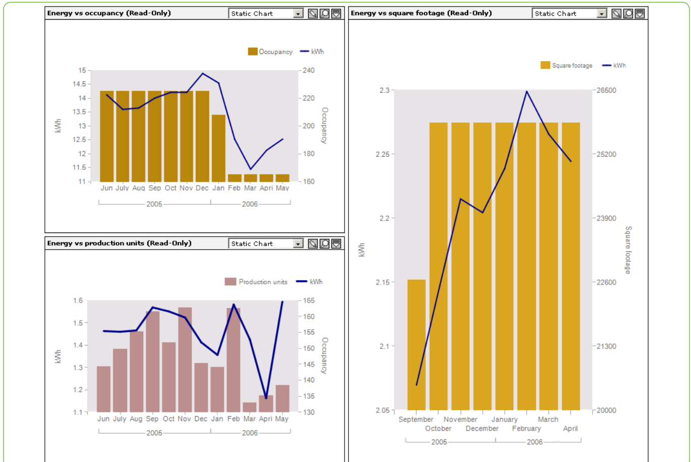
Figure 3 Example of EEM software with key performance indicators, benchmarking and normalization tools that help analyze and compare building performance and reveal opportunities to reduce costs.
